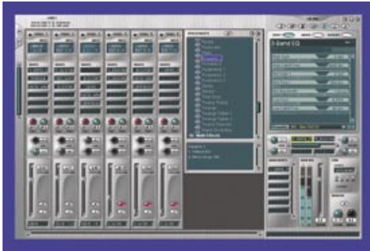
FIG. 2: The PatchMix console is home to Emulator X's DSP-based effects and also has an adaptive display of the channels that you have enabled.
