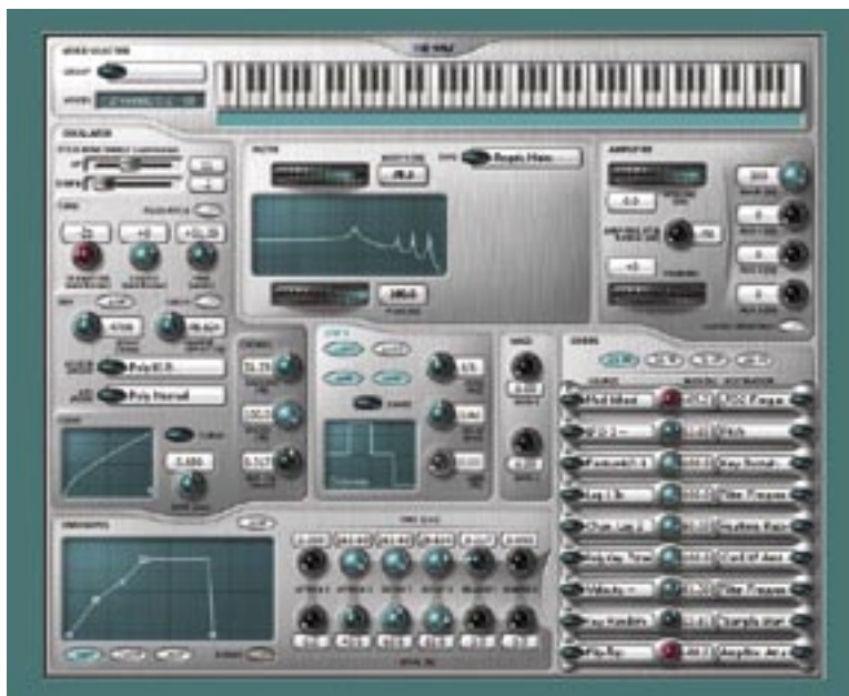
FIG. 5: The Voice-Processing screen is at the heart of the Emulator X's programmable parameters. You can save presets from each processing module.
