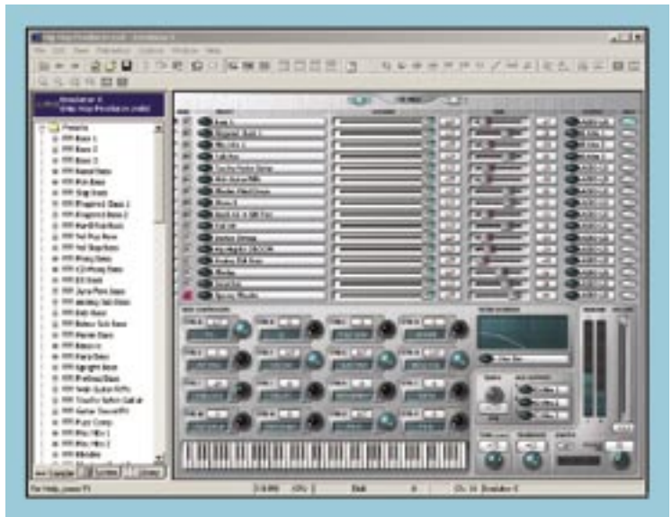
FIG. 3: Emulator X offers 32 MIDI channels, which you configure in the Multisetup screen. Any number of presets can be assigned to the same channel.
